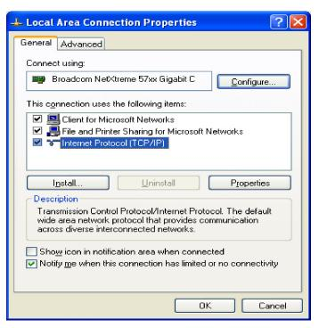
**Step 4:** On the Local Area Connection Properties page, double click on Internet Protocol (TCP/IP) to display properties.
