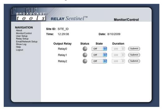
The Monitor/Control page allows the monitoring of each relay via each status LED. The relays may be configured for one of four states. OFF, ON, Pulse with selectable length of 100 to 2000 milliseconds and reboot with selectable duration of 1 to 30 minutes.
