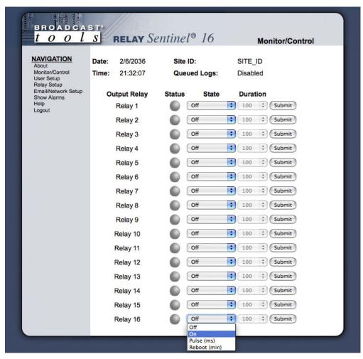
The Monitor/Control page allows the monitoring of each SS relay via each status LED. The SS relays may be configured for one of four states. ON, OFF, Pulse with selectable length of 100 to 2000 milliseconds and reboot with selectable duration of 1 to 30 minutes.
