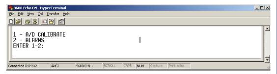
Select "1" to calibrate any of the analog (metering) inputs for the desired value. Selecting a "1" will produce the following prompt "Select Ch 1-4 followed by the desired 4 digit value". Enter the channel number, then the desired value.
