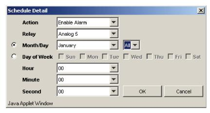
The Schedule Detail Dialog is used to set up a single schedule event. An event specifies an action (raise or lower), a relay or alarm muting/unmuting, and a time when the action occurs. The scheduler supports both day-of-month and day-of-week schedules. Wildcards can be specified in any of the date/time fields to create a repeating event.
