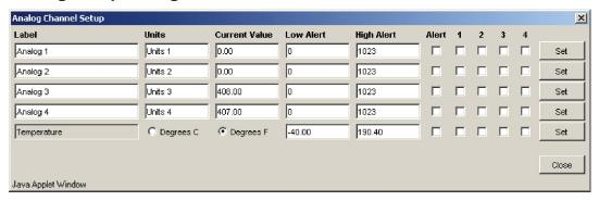
Analog Label Changes the label associated with any of the analog registers.
