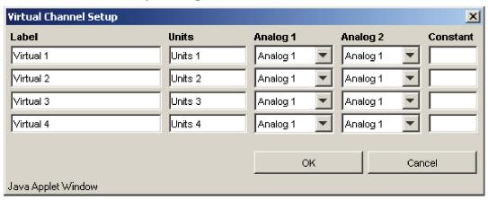
The WVRC-4 lets you define up to four "virtual" channels. These are similar to analog channels, but their values are derived from the product of two real analog channels and a constant.
