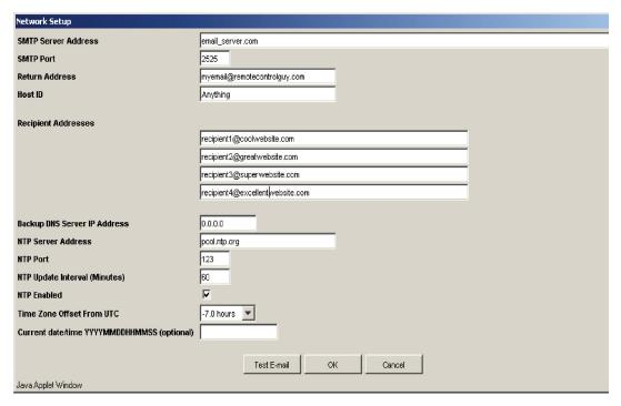
The Network Setup dialog allows the user to set up the following operating characteristics of the WVRC-4 firmware and applet.
