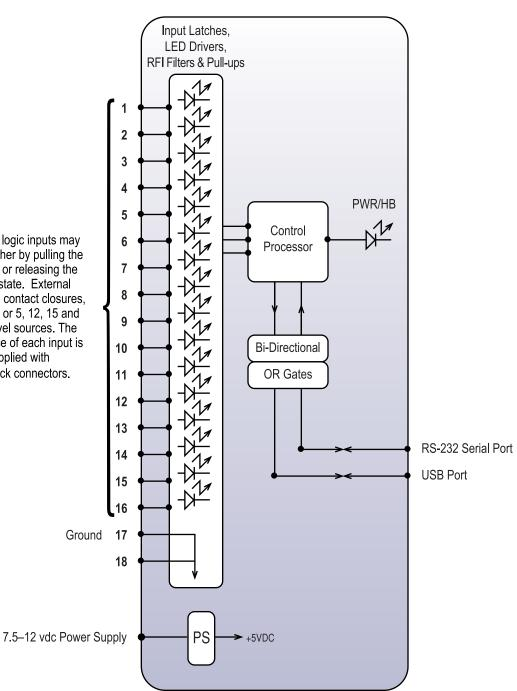
The 16 status / logic inputs may be activated either by pulling the input to ground or releasing the input to a high state. External sources can be contact closures, open collectors or 5, 12, 15 and 24-volt logic-level sources. The input impedance of each input is 22 K ohms. Supplied with Plug-in euroblock connectors.
