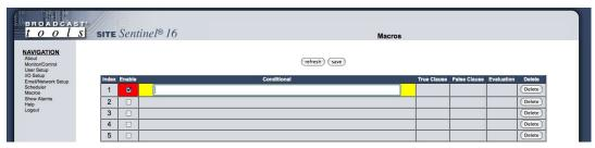
The Site Sentinel 16's macro system allows for the ability to trigger relay events based on combinatorial logic of status and meter inputs. Each of the 50 available macro slots has a conditional statement as well as a true and false clause. When a macro is enabled, it is evaluated every second and either the true or false clause is executed, empty true and false clauses are allowed and no action is taken if they are empty.
