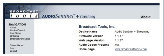
The "About" Web Page displays the product name, firmware version numbers, Audio Codec status (required for streaming functionality), and Broadcast Tools® Web site link.
