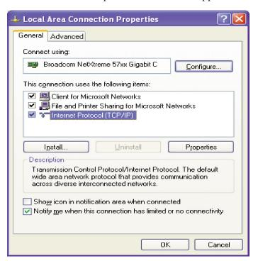
**Step 4:** On the Local Area Connection Properties page, double click on Internet Protocol (TCP/IP) to display properties.
