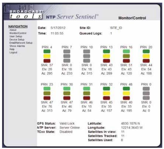
The Monitor/Control page provides an overview of the current status of the NTP server, and the GPS receiver. Allow at least 10 minutes for the receiver to get an initial location fix and acquire the required satellites for time sync.
