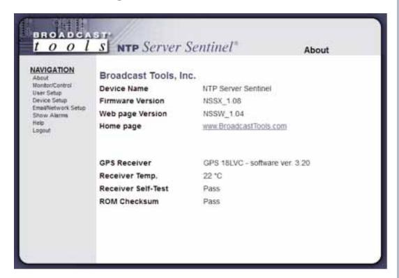
The "About" Web Page displays the product name, firmware version numbers, and Broadcast Tools® web site link. This page also contains version and diagnostic data for the connected GPS receiver.
