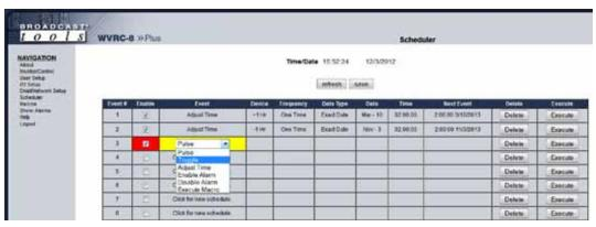
The Scheduler allows for complete control of your WVRC-8 Plus device by providing the ability to schedule when alarms are enabled or disabled, pulse or toggle relays, execute macros and even adjust the time for daylight savings.
