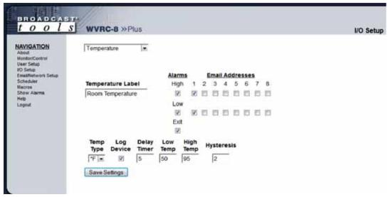
Temperature Label: Identifies the temperature input source.
