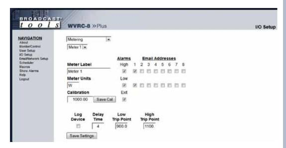
Metering input selection: Select metering inputs 1-8 for configuration. Meter Label: Used to identify the metering input source.
