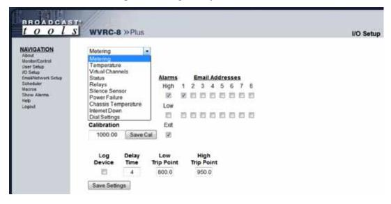
On the I/O Setup screen, choose from the top drop-down box the device to configure.
