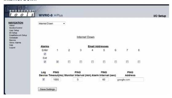
The Internet Down alarm allows the WVRC-8 Plus to monitor the reachability of a specified DNS address or IP address using an ICMP ping. The ICMP ping is a commonly used extension to the Internet Protocol (IP). ICMP supports packets containing error, control, and informational messages. The PING command, for example, uses ICMP to test an Internet connection.
