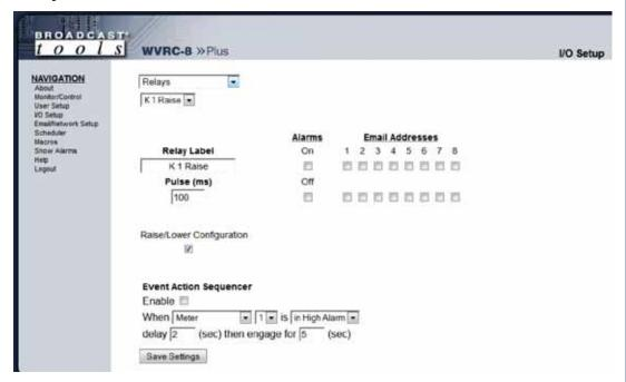
Relay Label: Used to identify the attached device/function.
