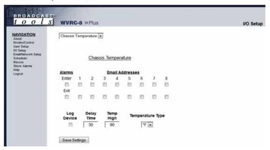
Alarms Enter: This option enables the "Temp High" alarm.
