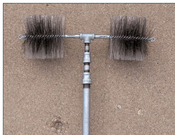
Add a few parts from the hardware store, and you can have a dual bleeder as shown.
